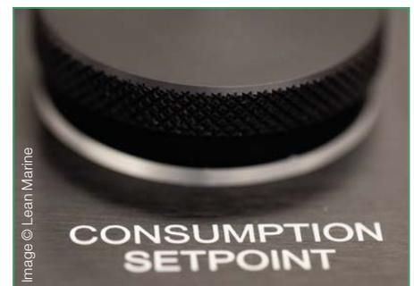
'FuelOpt controls the propeller's pitch and RPM separately in order to produce the most amount of propeller thrust with the least amount of power. This means less wasted energy – which in turn means less fuel consumption'
